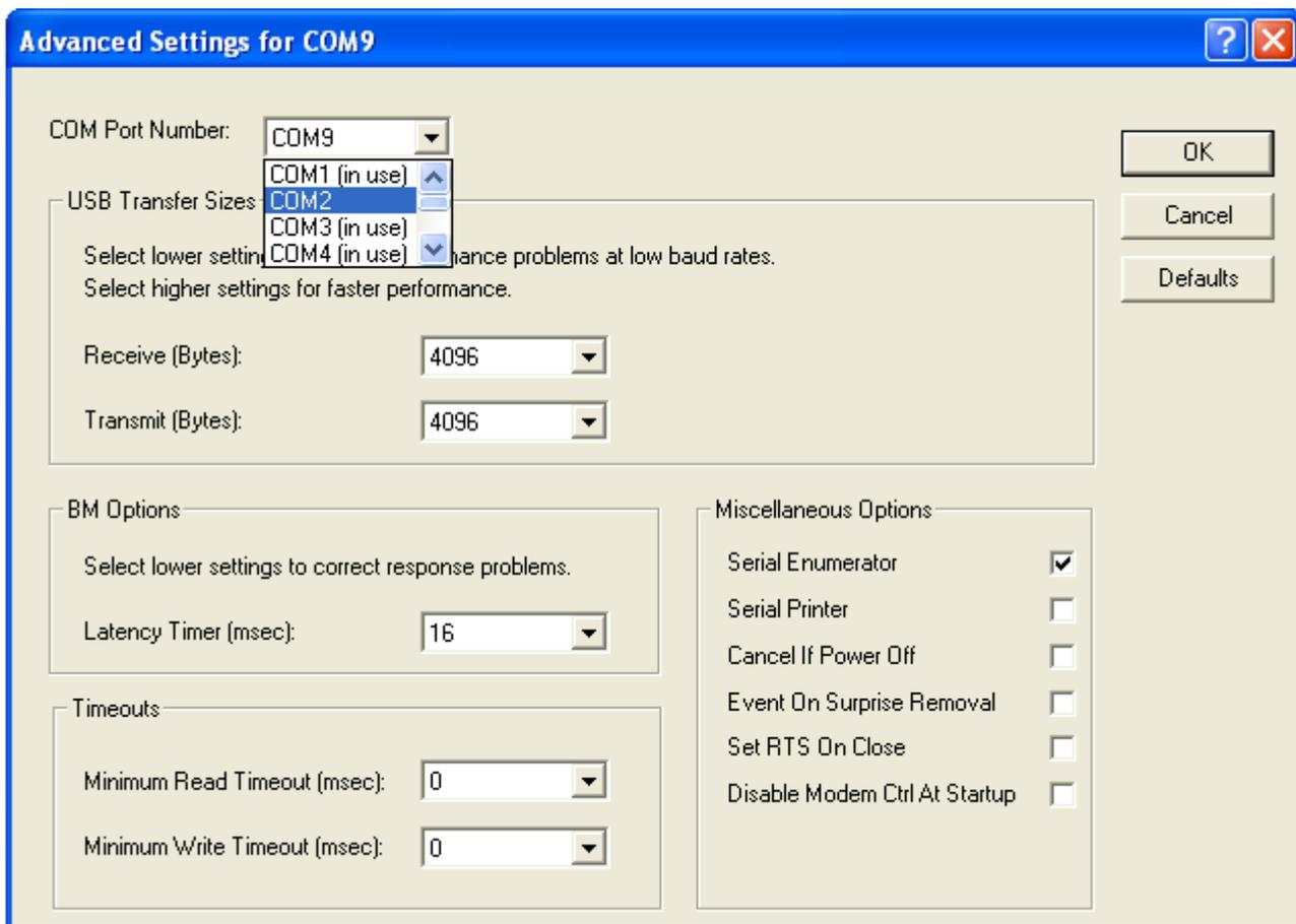
Confirm twice with **OK**. The settings are not updated immediately in the **Device Manager**. Close the **Device Manager** and start it again. The requested Com port should now be displayed.
