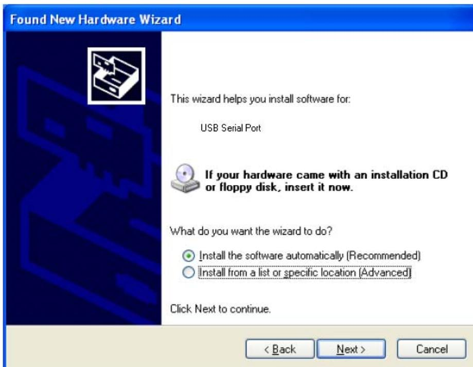
Select option ***Install the software automatically (Recommended)*** and confirm with **Next**.
